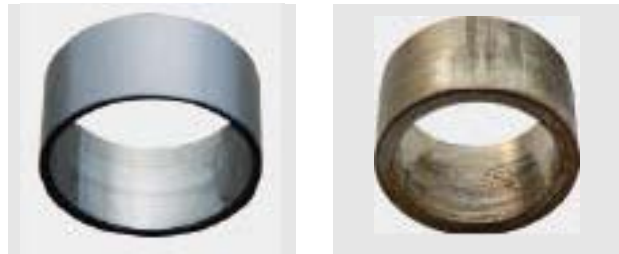
图表 2 塑料轴承与传统复合轴承的磨损 Graph2 Surface wear ( Plastic Bearing vs Metal bearing)
